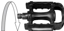
Right pedal: 'R' stamped on its axel indicates the right pedal. Tighten the screws in clockwise direction.
